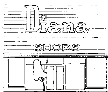
Inappropriate: sign obscuring upper story windows
