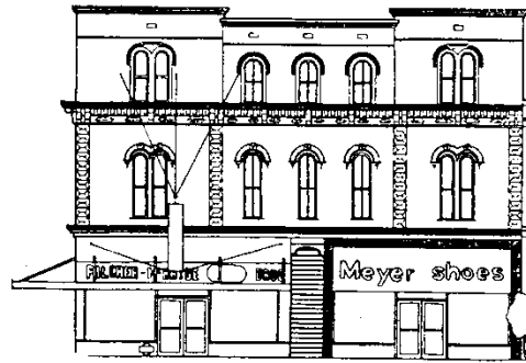
Inappropriate: removal of roof pitch
