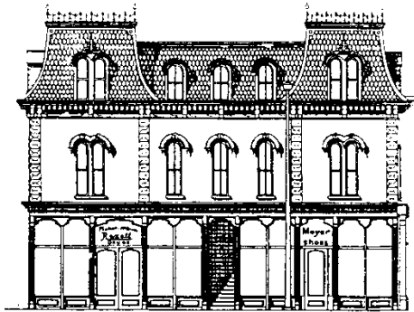
Appropriate: original mansard roof
