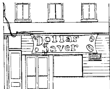
Inappropriate: sign and lettering too large for building
